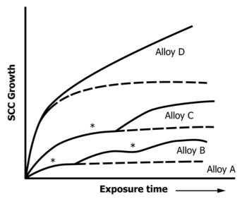
Note 1—Schematic of the influence of corrosion product wedging on SCC growth versus time curves in a decreasing K (constant displacement) test. Solid lines: actually measured curve for case of corrosion product wedging that results in increase in crack growth with time; asterisks indicate temporary crack arrest. Dashed lines: true crack growth curve excluding the effect of corrosion product wedging (9).
