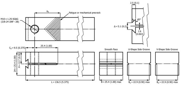
NOTE 1—All dimensions in mm (in.). Top and front views are shown for smooth specimen only; side view is shown for both smooth and side grooved configuration.
